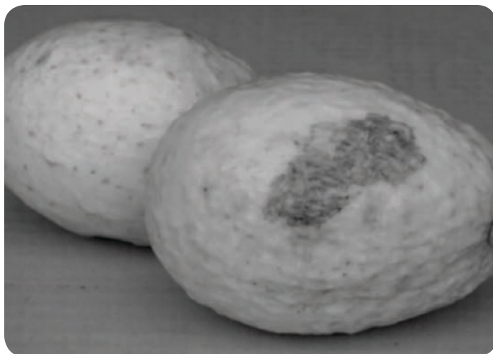
Figure 2: Infrared light through a filter highlights bruises on fruit.
