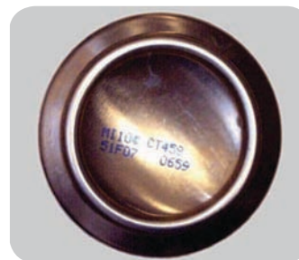
Figure 8a: A beverage can illuminated by direct lighting, in this case a ring light, reflects glare to the camera.
