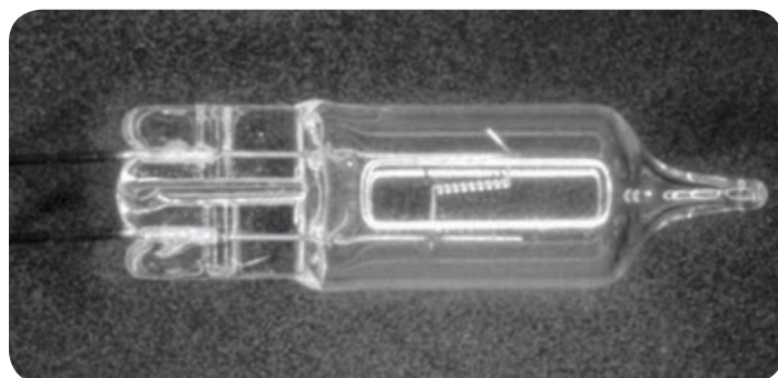
Figure 4a: Light bulb with direct illumination from a ring light. The ring light is reflected in the glass.
