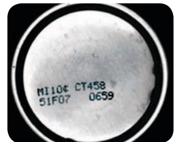
Figure 8b: The same can illuminated by diffuse off-axis lighting provides a clear image of surface markings.
