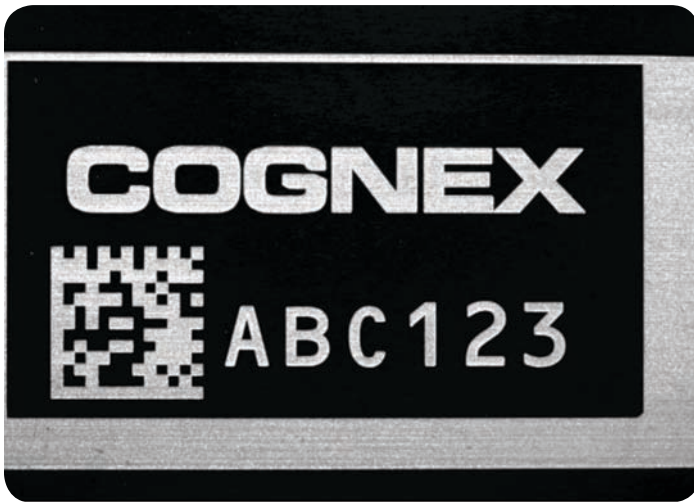
Figure 9a: Image taken of a moving part using strobe light illumination.
